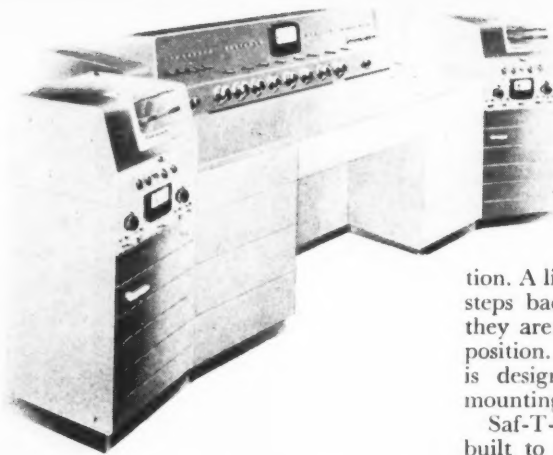
View of Finch "Printed Radio" Facsimile broadcast studio transmitter-monitor for FM broadcasters.
